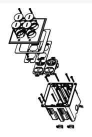
Includes dual-gang box, two 106 adapter with eight openings for communication devices, and nickel cover with four screw plugs. For hole cut dimensions, see installation instructions sheet. Box Dimensions: 3 1/4" W x 3 3/4" L x 3 7/8" D (83mm W x 95mm L x 98mm D) Device Plate: 4.7/8" W x 5 1/16" L (124mm W x 129mm L).
