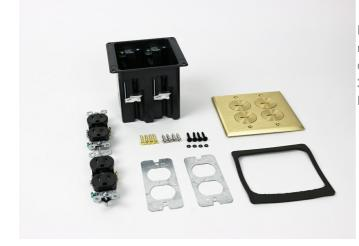
Includes dual-gang box, two 15A tamper-resistant duplex receptacles, and brass cover with four screw plugs. For hole cut dimensions, see installation instructions sheet. Box Dimensions: 3 1/4'' W x 3 3/4'' L x 3 7/8'' D (83mm W x 95mm L x 98mm D) Device Plate: 4 7/8'' W x 5 1/16'' L (124mm W x 129mm L).
