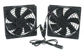
Fan kits for the Vertical Wall-Mount include (2) 115VAC fans, power and grounding cord, fan guards, and hardware. Fans deliver 85CFM each. Proved active cooling for wall-mount cabinets.
