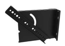
Vertical Wall-Mount fixed 8RU adjustable mounting rail kit. 8RU only mounts into the 8RU frames. The mounting rails can mount equipment using 10-32 hardware, or can be reversed to mount using cage nuts in any thread size.
