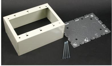
Designed especially for use in the installation of signal system and alarm wiring. Base has 1/2" trade size KOs. Larger gang boxes available by special order. Threegang: 4 5/8" L x 6 1/2" W (117mm x 165mm). NOTE: Certified to Canadian Safety Standards for sale in Canada. When ordering these products, change the "V" color prefix to "vc" or the "WH" color suffix to "WHC" to denote the Canadian versions.
