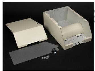
Feeds 2400 and 2400D Series Raceway. Has 1/2", 3/4", and 1" trade size KOs on back and end. Removable divider and radiused insert included.
