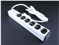
20A configuration. Four outlets, white finish. 15' (4.6m) cord. Length 10 3/4'' (237mm). Receptacle center-to-center 1 1/2'' (38mm). cTUVus Listed as Medical Electrical Equipment. Suitable for use where Article 517 of the NEC requires Hospital Grade Outlets.
