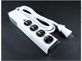
Four outlets. Rugged white aluminum housing. 6' (1.8m) 14/3 SJT white cord with NEMA5-15 plug. Length 10 3/4'' (237mm). Receptacle center-to-center 1 1/2'' (38mm). Snap-on, slide-off mounting. Not for use in critical care enviornments. NOTE: Not for use where Article 517 of NEC requires Hospital Grade Outlets.
