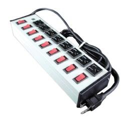
Eight individually switched outlets, lighted on/off switch, putty white finish aluminum housing, 15A. 6' (1.8m) 14/3 SJT black cord with NEMA5-15 plug. Length 13'' (330mm), width 3 1/2'' (89mm). Receptacle center-to-center 1 5/16'' (33mm). Snap-on, slide-off mounting.
