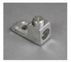
For use with SpecMate or Cablofil brand cable trays to provide ground continuity. Electroplated aluminum. Dual rated for copper and aluminum conductors, No. 2 to 14 gage cable.
