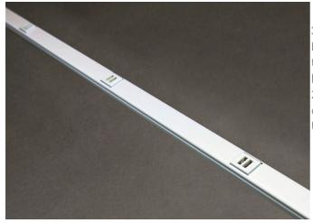
3' (914mm) length with 12'' spacing. USB is 2.4 Amps (shared between two ports) 5VDC. .040'' (1.0mm) steel housing. Packed two per carton. Each unit supplied with one (1) Coupling and two (2) Blank End Fittings. Each USB module provides 2 ports with 2.4 Amps of shared charging. Please note the charging load on one module will not affect the charging performance of the other USB modules in the product.
