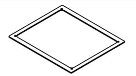
Used for floor coverings greater than 1/4" (6.35mm). Use one spacer for 3/8" (9.53mm) thick tile. Use two spacers for 1/2" (12.70mm) thick tile. The RFB119-TS will allow the top surface of the cover assembly to be flush with 3/8" (9.53mm) to 1/2" (12.70mm) floor coverings.
