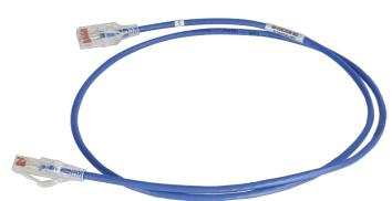
RDC 6 Modular Patch Cord, blue, 9', reduced diameter, 28 AWG, cat6 channel four-pair UTP stranded PVC/CM.
