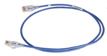
RDC 6 Modular Patch Cord, blue, 5', reduced diameter, 28 AWG, cat6 channel four-pair UTP stranded PVC/CM.
