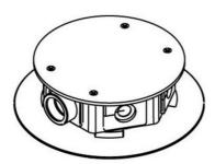
Complete with gray or black carpet flange, gray hexagonal housing, five black rubber grommets, and one 3/4" trade size threaded dropin hub. The service head includes scrub water gasket. Colors available in painted gray (GY), and black (BK). Use with the RC9FFS Insert to form a complete poke-thru assembly. NOTE: RC9AFFTC Series Poke-Thru Devices require a 3" (76mm) diameter hole. Not designed to work with bare concrete or terrazzo. Floor covering thickness 1/8" minimum.
