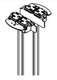
Prewired snap-in 20A receptacle with 25' (7.62m) leads, can be wired as standard duplex or isolated ground. Available only in black. See installation instructions with replacement receptacle for complete installation details.
