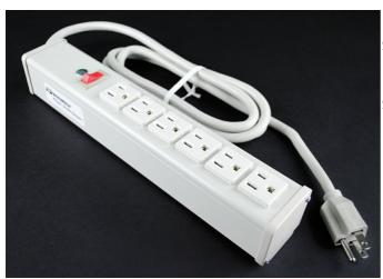
Six outlets, putty white aluminum housing, 15A, lighted switch. 15' (4.6m) 14/3 SJT putty white cord with NEMA5-15 plug. Length 12 1/4'' (311mm). Receptacle center-to-center 1 1/4'' (32mm). Snap-on, slide-off mounting.
