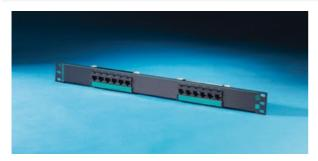
Clarity 5E 12-Port Patch Panel is component compliant to EIA/TIA Category 5e performance requirements. Standard density design provides additional space for cabling and occupies one rack unit, measuring 19" x 1.75". Jacks are grouped in six-port modules. Part of the Clarity 5E link and channel solution that provides significant installed performance headroom.
