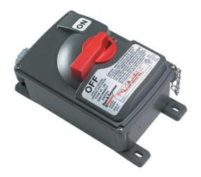
Non-Fusible Safety Switch with Auxiliary Contact, 60 Amps, 600 VAC. The first non-metallic NEMA 4X Non-Fusible Safety Switch line UL Listed as Suitable as Motor Disconnect per NEC Article 430.109(A) (6). Pass and Seymour Non-Fusible Safety Switches feature extratough components, including an impact-resistant Valox NEMA 4X enclosure. And an innovative design that delivers safe, sure operation under the worst conditions.
