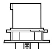
4-Pole, 5-Wire, Pin and Sleeve Inlet. 20A, 3Y, 120/208V.
