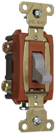
Canadian 3way Switch, Back & Side Wire, 20amp 347volt, Gray
