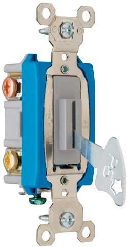
3-Way Lock Switch, Back and Side-Wire, 15A 120/277V (Key can be removed in both positions)
