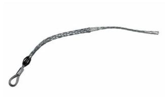
Medium Duty, Standard Length, Flexible Eye, T-Type. Cable Diameter - 2.500-2.990-inch, Mesh Length - 36-inch, Eye Diameter - 1/2-inch, Break Strength - 24,500 lbs.
