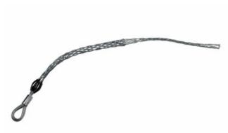
Medium Duty, Standard Length, Flexible Eye, T-Type. Cable Diameter - 2.000-2.490-inch, Mesh Length - 36-inch, Eye Diameter - 7/16-inch, Break Strength - 18,500 lbs.
