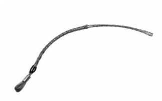
Medium Duty, Standard Length, Flexible Eye, T-Type. Cable Diameter - 1.500-1.990-inch, Mesh Length - 36-inch, Eye Diameter -7/16-inch, Break Strength - 16,400 lbs.
