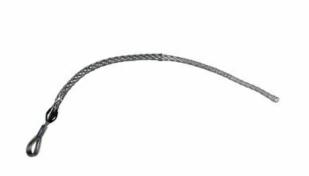
Medium Duty, Standard Length, Flexible Eye, T-Type. Cable Diameter - 1.000-1.490-inch, Mesh Length - 36-inch, Eye Diameter -5/16-inch, Break Strength - 9,600 lbs.
