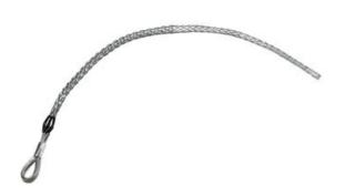
Medium Duty, Standard Length, Flexible Eye, T-Type. Cable Diameter - 0.750-0.990-inch, Mesh Length - 36-inch, Eye Diameter - 1/4-inch, Break Strength - 6,800 lbs.
