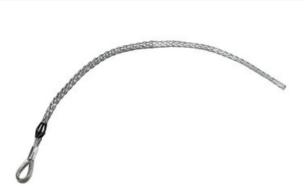
Medium Duty, Standard Length, Flexible Eye, T-Type. Cable Diameter - 0.750-0.990-inch, Mesh Length - 36-inch, Eye Diameter -1/4-inch, Break Strength - 6,800 lbs.
