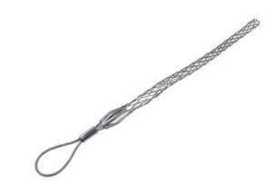
Light Duty, Short Length, ◆ Flexible Eye. ◆ Cable Diameter - 1.000-1.240\'\', Mesh Length - 14\'\', Break Strength - 5,800 lbs.
