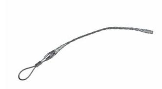
Light Duty, Standard Length, ◆ Flexible Eye. ◆ Cable Diameter - 0.620-0.740\'\', Mesh Length - 16\'\', Break Strength - 4,100 lbs.
