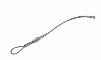
Light Duty, Short Length, ◆ Flexible Eye. ◆ Cable Diameter - 0.620-0.740\'\', Mesh Length - 11\'\', Break Strength - 4,100 lbs.
