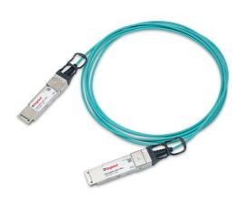
3m Palo Alto PAN-QSFP-AOC-3M Compatible 40GBase-AOC QSFP+ to QSFP+ (MMF, 850nm, LSZH) Active Optical Cable
