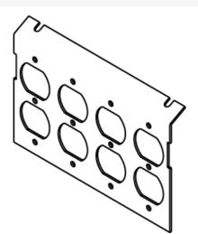
Four [4] duplex KOs. One plate supplied with AC8850 Box. NOTE: AC8850 is a single-service box. Power plates cannot be used in conjunction with communication plates.
