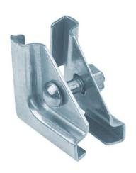
Clamps are used to junction runway sections together in a variety of configurations. Whether sections are extended in-line or junctioned perpendicularly or are transitioned from horizontal to vertical, clamps provide a solid connection to assure the runway layout will provide the necessary support for your cabling.
