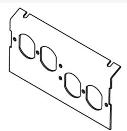
Two (2) duplex KOs. One (1) plate supplied with AC8104 Box. NOTE: AC8840 is a single-service box. Power plates cannot be used in conjunction with communication plates.
