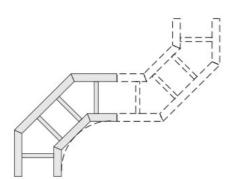
For extremely corrosive applications we offer a full line of straight sections, fittings, covers and mounting accessories in polyester and vinylester fiberglass. Rail heights are available in 4" and 6" and widths are available up to 36".
