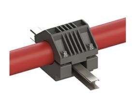
Cablofil cable cleats are designed to restrain cables from lateral and torsional forces supported by ladder tray. In vertical applications, cable cleats provide axial strain relief to cables without damaging the cable sheath. Cablofil heavy-duty cable cleats enclose the cable and the ladder rung with a rigid hi-strength interlocking frame that protects high, medium and low voltage cables from mechanical damage resulting from short circuits.
