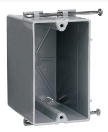
Single-Gang, Deep Switch and Outlet Box, Reverse Angled captive Mounting Nails on Each End, Two Quick/Click Entries on Each End. Extra deep for dimmers, GFCIs and thermostats, yet suitable for 2x4 construction. 100 pack.
