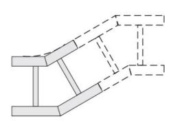
Choose from an extensive selection of metallic ladder tray with a variety of rung and bottom styles to choose from. Finishes include steel, 304L and 316L stainless steel to meet the needs of any application. Rail heights range from 4" to 7" and width sizes are available up to 36".
