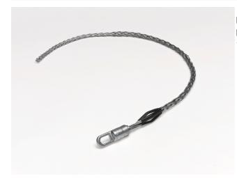
Multi-Weave, Rotating Eye. Cable Diameter - 0.750-0.990-inch, Mesh Length- 41-inch, Eye Diameter - 1-inch, Break Strength -14,400 lbs. Light Blue.
