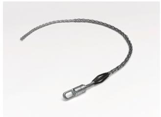
Multi-Weave, Rotating Eye. Cable Diameter - 0.750-0.990-inch, Mesh Length- 41-inch, Eye Diameter - 1-inch, Break Strength - 14,400 lbs. Light Blue.
