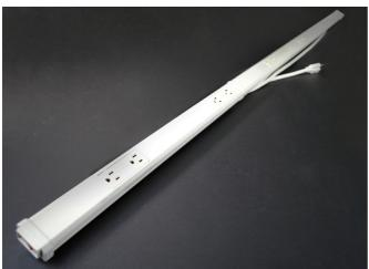
Twelve (6 duplex) outlets, nonmetallic housing with ivory finish. 6' (1.8m) cord. Length 48'' (1.2m). Receptacle center-to-center 12'' (305mm).
