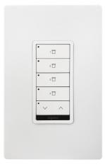
LMSH-SW2xx Series Wall Switches are low voltage devices for manual control of shades from one or more locations. They are part of a Digital Lighting Management (DLM) system and can control any shade motors connected to DLM shade controllers
