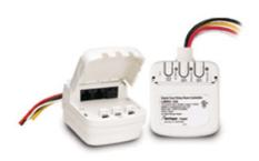
LMRC-100 Series Digital Room Controllers include one or two relay(s) for on/off control of a total of 20 amps, and a highefficiency switching power supply. They are the foundation of a Wattstopper Digital Lighting Management (DLM) system, and allow integration of occupancy sensors, daylighting sensors and switches for energy-efficient lighting control.
