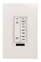
The LMPS-104 Digital Partition Switch enables quick manual coordination of lighting controls in flexible spaces with up to four movable walls. It is part of a Digital Lighting Management (DLM) system, and can reconfigure connected switches and occupancy sensors. The LMPS-104 may also be used as a status indicator when an LMIO-102 Digital Partition Interface is used for automatic coordination of controls.
