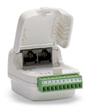
The LMIO-201 Analog Sensor Input Module is a single channel low voltage analog sensor to Digital Lighting Management (DLM) interface. It communicates a single state of occupancy, however it may be driven by multiple physical sensors wired together. The LMIO-201 works in conjunction with an auxiliary DC power source.
