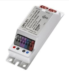
The LMFC-011 fixture controller mounts in individual lighting fixtures to give them connectivity to a Digital Lighting Management (DLM) system. The controller provides a 0-10 volt signal for control of dimmable loads including compatible LED drivers and electronic ballasts and connects to the DLM local network via a single- or dual-port RJ45 wiring whip (ordered separately). Each DLM local network can support up to 64 loads.
