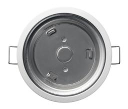
The LMDL-600 is a wireless open loop photo sensor that measures the daylight contribution in order to automatically switch or dim multiple zones of lighting. It is part of the NEW wireless Digital Lighting Management (DLM) system and sends light level signals to control loads connected to DLM on/off or dimming room controllers.
