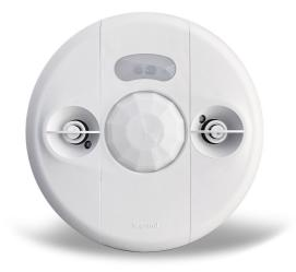
The LMDC-100 low profile Dual Technology Ceiling Mount Occupancy Sensor uses both passive infrared (PIR) and ultrasonic technologies to achieve precise occupancy sensing for energyefficient control of lighting and plug loads. It is a digital sensor, and is part of a Wattstopper Digital Lighting Management (DLM) system.
