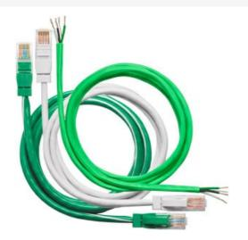
This type of wire connects low voltage devices (i.e., switches, occupancy sensors, photocells) to panels. It is #20 AWG wire that meets UL and NEC standards for Class 2 applications. Plenum rated wire meets plenum and riser requirements. Several types of multiconductor low voltage wires are available for standard, pilot, locator, and multilevel switching or for connecting photocells to the LI control panels. This wire can also be used to wire relays remotely
