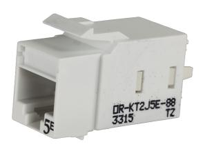
Category 6 Keystone jack, 8-position, 180 degree exit, icon compatible, T568A/B wiring, White , individually packaged. Keystone, KT2J jacks and modules feature New installer friendly lacing cap termination with free termination tool in every carton. The keystone footprint allows flexibility in installation scheduling because its rear insertion into the faceplate allows the technician to complete the termination before and during the construction process.
